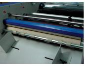
The adjustable burster automatically separates sheets up to B2 size. A cushion of air supports the sheet as it is delivered into the catch tray.
