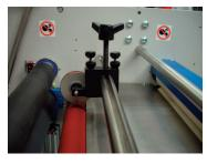
The positioning of the perforator overcomes any potential issues caused by poor film roll profiles and allows higher speeds to be maintained.
