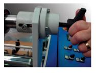
The madrel has a hinged support and film can be adjusted laterally on the run to minimise waste and down time.
