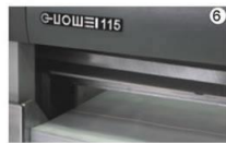
光学对刀线, 使裁切更方便 The optical knife alignment make cutting more convenient.
