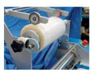
A film slitter is provided to allow non-standard sheet sizes to be run when using a wider standard width film, reducing the need to carry stocks of non-standard film widths.
