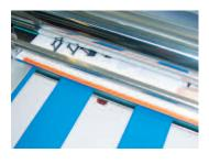
A 'missing sheet' detector stops the laminator if no sheet is detected helping to avoid messy wraparounds.
