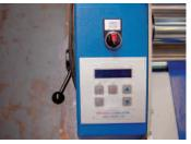
A simple control panel allows speed and temperature to be adjusted to suit the work being run.
