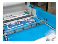
The automatic sheet separator is adjustable to separate any size of sheet up to B2 and allows the laminator to be run by a single operator.
